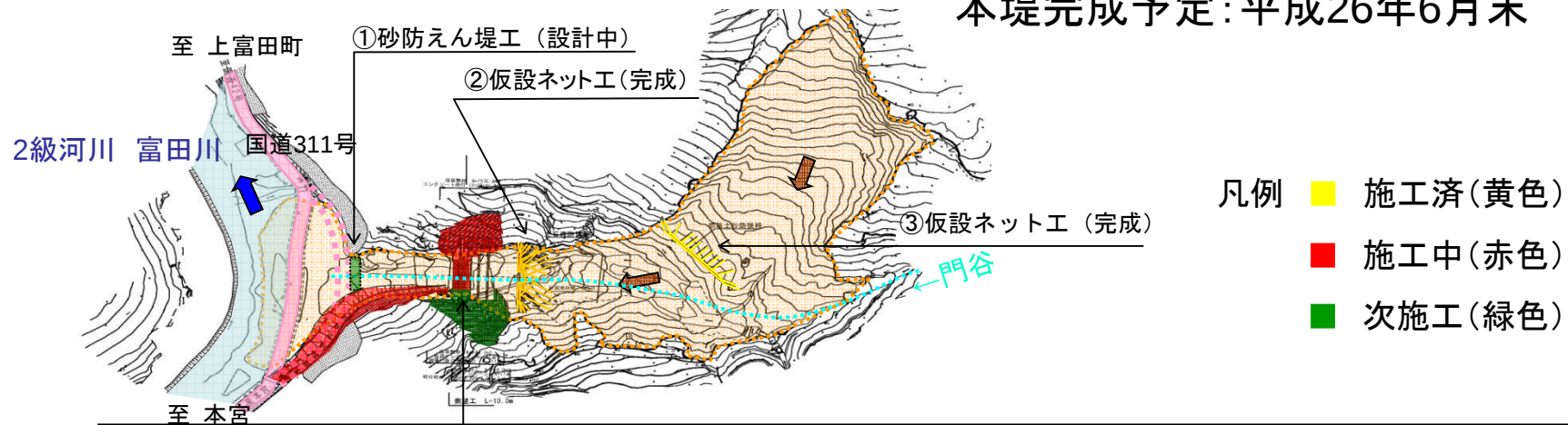
①砂防えん堤工 (H=14.5m, L=59.5m)
